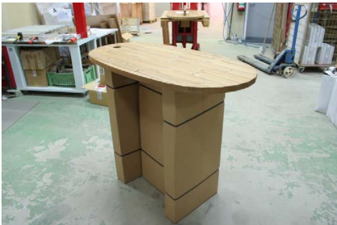
Bottom is placed on three boxes. With the assembly line facing upwards.
