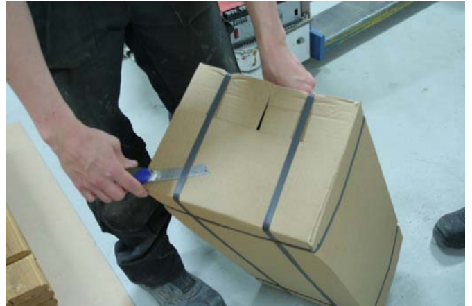
Open the boxes by cutting only the longer straps, leave the others because the boxes will serve as an assembly table.
