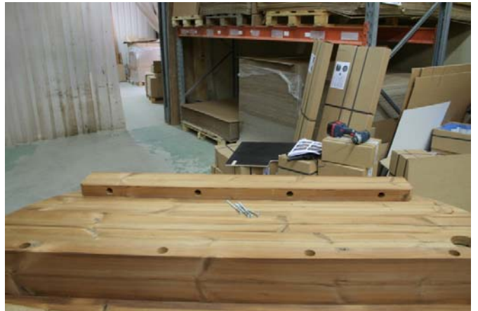
Assemble the support legs first, there are pre-drilled holes where they are to be fastened.
