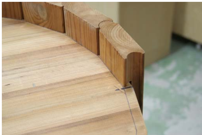
Begin with the first stave at the marked position. See picture to the right for more information.
