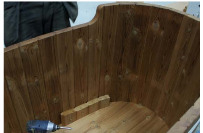
Fasten all the pieces in the side as the picture shows. NOTE! The first and last piece are not identical, see picture. Repeat the procedure for the other side.
