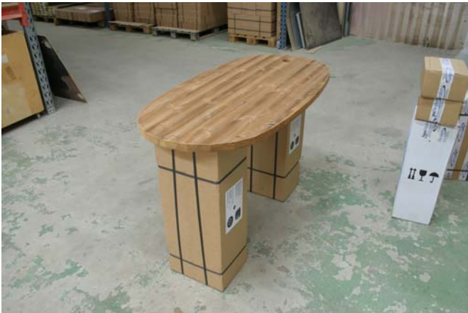
Bottom is placed on two boxes. With the assembly line facing upwards.
