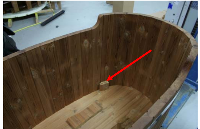
Place the first support piece at the fifth stave as the arrow indicates. See picture 2 on the last page for more information.
