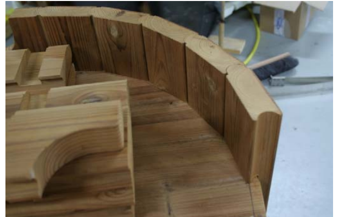
WRONG! The staves are crossing the line!
