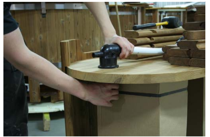
Use the included tool to screw the drainage valve in place.
