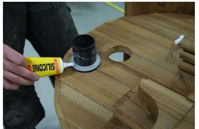
Now is also a good time to assemble the drainage valve. Apply silicone on the threads.
