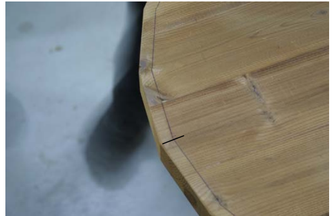
Begin with the first stave at the marked position. See picture 1 on the last page for more information.
