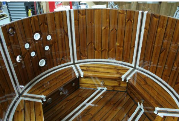
4. Apply masking along the innermost black line on the seating well.
