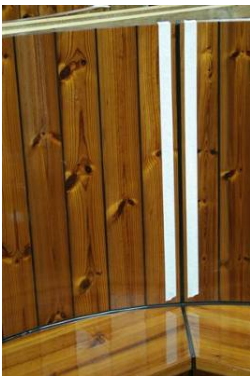
5. When the side modules are assembled and the sealing mass has dried for at least 6 hours, the vertical joints and the joint between the seat and side should be coated using the method illustrated earlier. Let it dry for at least 12 hours before checking for leakage. If the application of coating is made after the bath has been in use then the coating should be applied only after the joints, and a small area out from this, are cleaned with acetone and sanded.
