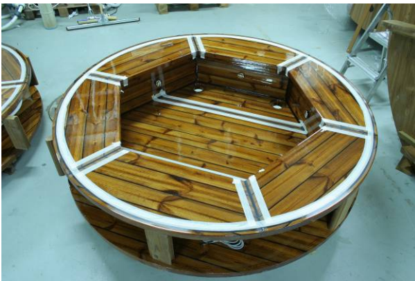
4. Apply masking along the innermost black line on the seating well.
