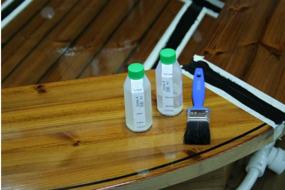
1. The coating consists of two components, "Comp. A" and "Comp. B", the mixing ratio is 4:1 (A:B)
