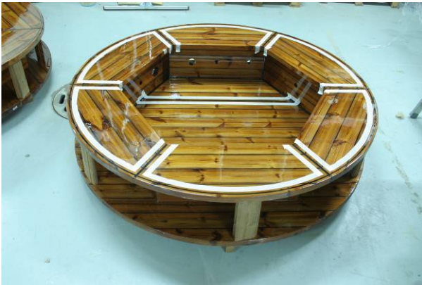
3. Apply new masking at the outer edges, following the same line as before.
