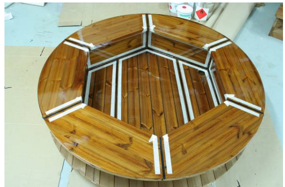
4. Turn the seating area and apply coating onto the joints between the seats and the two joints in the base. Remove the tape afterwards. Wait 5 hours and then apply new masking, sanding and plastic application according to "second coating"
