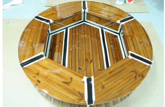
2. In order to get a good looking result the masking is applied "double". See "Mask properly". Remove the masking tape for the joints. Let it dry for at least 6 hours before
